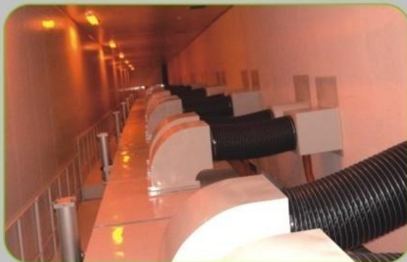
輥式烘箱 Roller type drying oven
