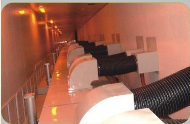
輥式烘箱 Roller type drying oven
